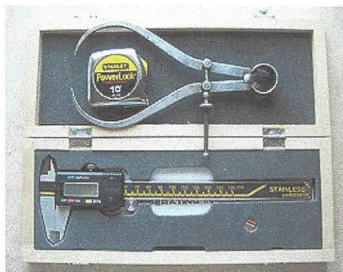
Three tools for measuring the diameter of solid shot: the diameter tape, the machinist's feeler gage and the electronic caliper.
