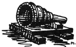
FIGURE 4—EARLY SMALL BOMBARD (1330). It was made of wrought-iron bars, bound with hoops.
