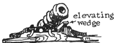
FIGURE 36—BRITISH MORTAR ON ELEVATING BED (1740).
